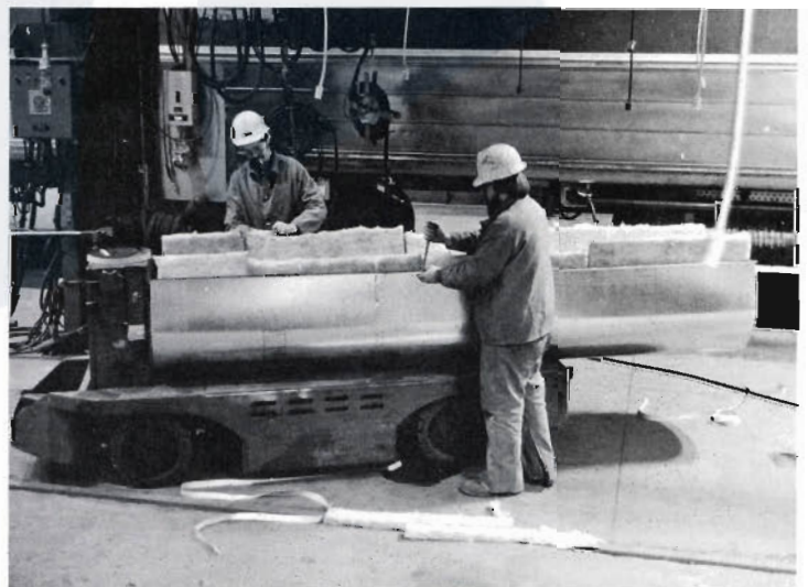
(Left) Charles Mitchell, machinist, creates some brass nuts on a shop lathe. (Above) Tom Leathers, carman, and John Skaggs, carman-welder, assemble a foam-lined jacket for covering and insulating a car's water tank.
