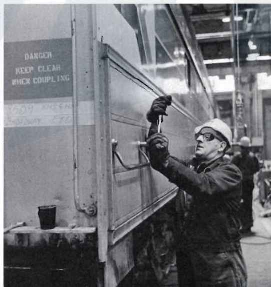
(Below) Dave Kern, carman, connects heating elements along the floorboard.
