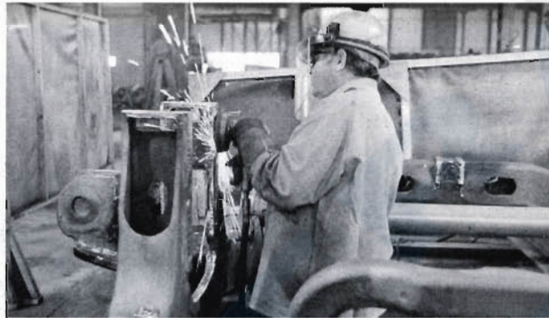
(Above) A welder works on the end bulkhead of a car. (Upper Right) J.S. Nowosielski, machinist, repacks bearings that will be used in reassembled trucks. (Right) Chester Hollis, carman, grinds down some rough spots on a truck frame.
