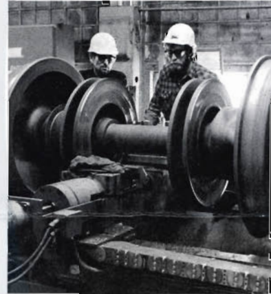
(Above) Julius E. Trageser, machinist, and John P. Callahan, machinist apprentice, face off a disc for an Amfleet wheel set on the Farrell axle lathe.
